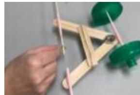
i. Attach the right front wheel. Turn the car sideways so that the assembled wheel is on the ground, then slide the axle through the straw. Add the second front wheel using hot glue, and flip it so that the glue doesn't connect to the straw on the frame. Make sure that the straw remains fixed, but that the axle will spin inside the straws.
