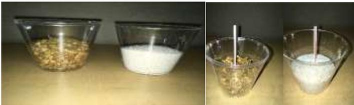
3. Predict and test porosity by making puddles: How much water you think each aquifer can hold? Write it down.
