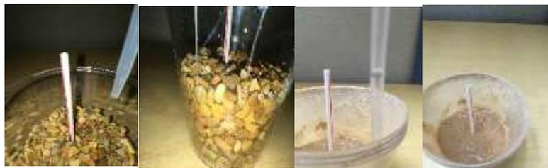
Measure water in your graduated cylinder. Write down how much you start with. Use the dropping pipet to “rain” drops of water along the surface of the aquifer. Watch the water percolate (infiltrate) through the pockets of air. Then when the entire aquifer is filled, and all the pores are saturated with
