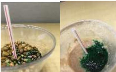
5. Remove the pollution through the well: Use the dropping pipet to carefully suck out/remove water from the well. Measure how much water must be removed before the food coloring shows up. The faster the pollution moves through the aquifer, the higher the **permeability**, or connectedness of the pore spaces.
